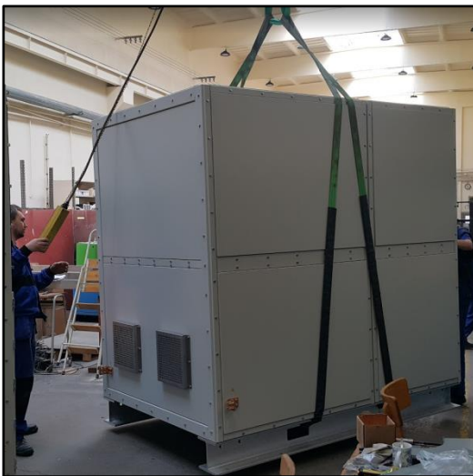
Examples of lashing and lifting the switchboard cabinets
