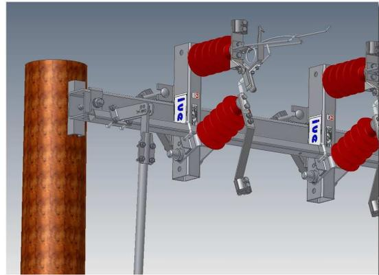
**IX. Flexible flag contact** – eliminates excessive stress and bends acting on the cables or conductors. The flag contact is terminated with the KG43 clamp and can be mounted at a later time to the basic version of switch disconnector.
