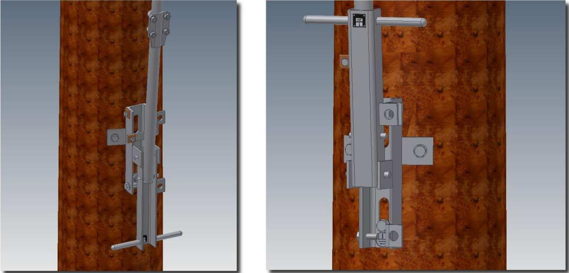
**II. Connecting rod guides** - these support the connecting rods along the wooden pole when operating the switch and prevent excessive cambering of the connecting rods during the handling operations. The guides are fixed to the pole using wood screws. Also rod guides can be suitable for montage on an other types of poles.
