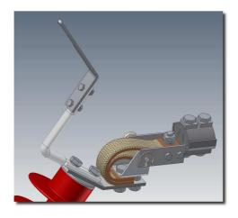
**X. Third supporting insulator** – if such is used it establishes a fixed connecting point on the switch disconnector and its purpose is to eliminate any stresses acting on the incoming power cables during the switch disconnector operations. The installation of the insulator to the switch disconnector can be done at a later stage.
