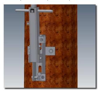
**II.** Connecting rod guides - these support the connecting rods along the wooden pole when operating the switch and prevent excessive cambering of the connecting rods during the handling operations. The guides are fixed to the pole using wood screws. Also rod guides can be suitable for montage on an other types of poles.
